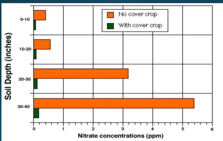
Figure 3. Effect of a cereal rye cover crop on soil nitrate concentrations (ppm) in broccoli plots fertilized the previous spring with 250 pounds Nacre. Samples were taken April 15, 1992.
